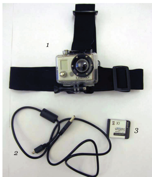
Figure 1. Headcam (GoPro® Hero HD) used in our research projects. 1 = video camera with head band, 2 = cable for downloading video files, 3 = extra battery.
